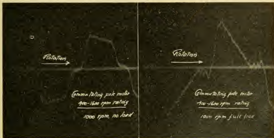
FIG. 294.—These films are for the same motor as used in getting Fig. 293; the speed is here 1000 r.p.m. and the main field is about one-third as strong as it was when getting Fig. 293. The field is much more distorted than it was with the strong field used for the speed of 400 r.p.m.
